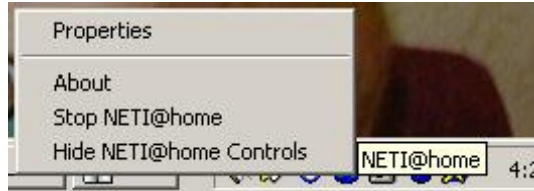
Figure 2: Screenshot of the NETITray menu. From this menu, users are able to select between the Properties window (Figure 3), the About window, an option to halt NETI@home’s collection of measurements, and an option to close the NETITray application.
